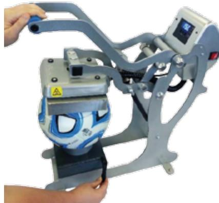
3. Using the handle to raise or lower the Ball Mount will adjust print pressure. Most balls will print well with about 5cm of space between the Electromagnet and the steel plate on the handle.
