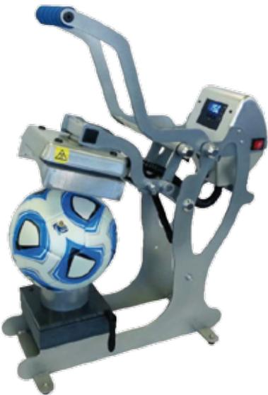
2. Lower the handle until the heater touches the ball, then unlock the Ball Mount by rotating the Adjustment Handle counter-clockwise.
