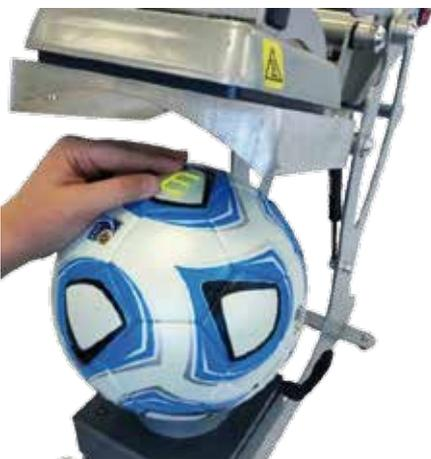
5. Lower and lock the handle to print. The timer will count down and automatically raise the heater when the press cycle is complete. When the handle lifts, the timer will re-set and you are ready for the next application.
