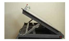
**Step 1**Adjust your Weeding Table to one of the 3 elevated heights, by lifting the outside edge of the table and tilting. Be sure the crossbar is secure before releasing.
