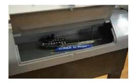
**Step 3**The Weeding Table comes equipped with a storage compartment on the front of the unit
