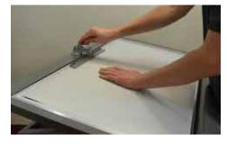
**Step 2**Secure medio to the Weeding Table using the material hold down bracket or simply place material on top of the table.
